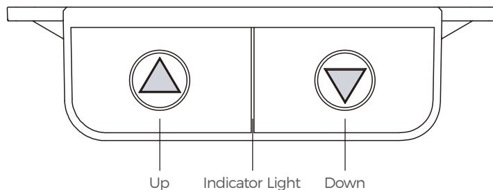
For the first use, press and hold the "↓" button until it moves to the lowest position and beeps. After, it can be raised and lowered normally.
